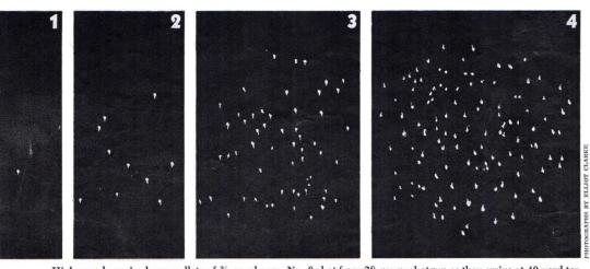
High-speed movie shows pellets of  $^{3}4$ -oz.-charge, No. 6 shot from 28-gauge shotgun as they arrive at 40-yard target. Left: First pellet strikes lead-foil screen. In less than 1/100 of a second complete shot charge has arrived.
